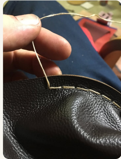
Stitching the leather to the bellows cheek: the leather meets the edge.
