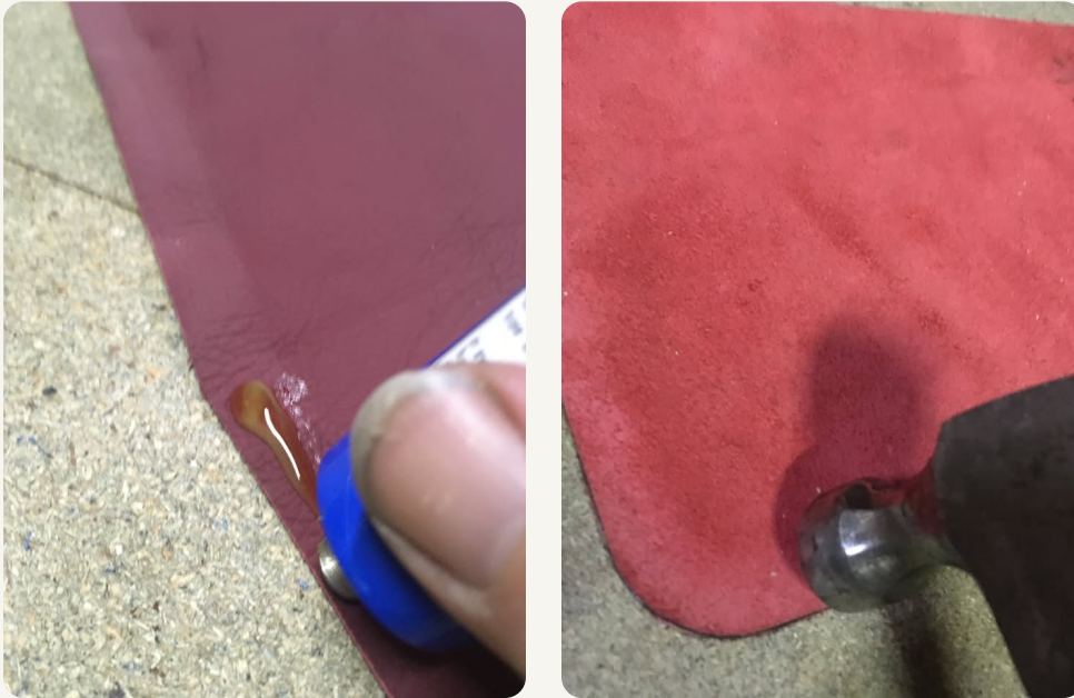
Applying cement, then lightly hammering the joined leather edges.
